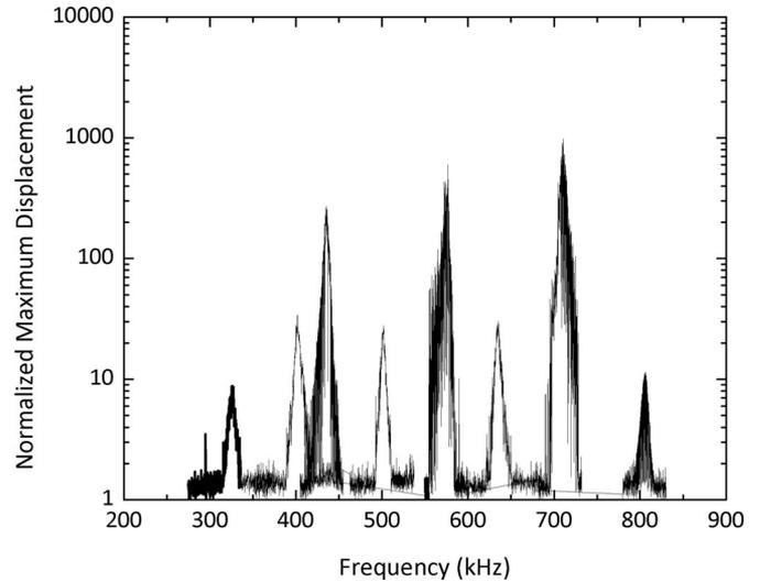
Fig. 8. The frequency response of a family of eight resonators with different geometries and resonant frequencies.
