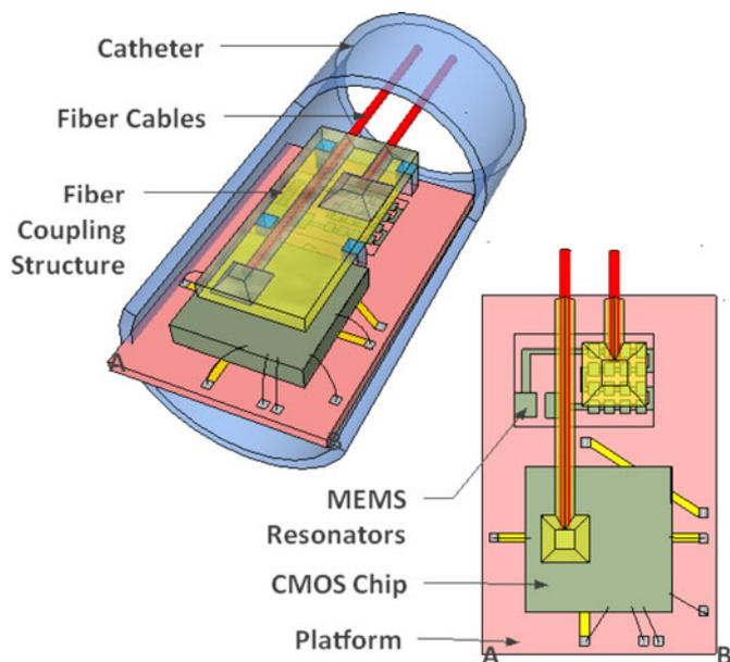
Fig. 1. General representation of the tracking microsystem fit in a catheter.
