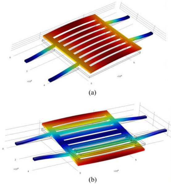
Fig. 3. Mode analysis simulations of a resonator. (a) Out-of-plane mode ( $f = 325$  kHz) and (b) torsional mode ( $f = 379$  kHz).
