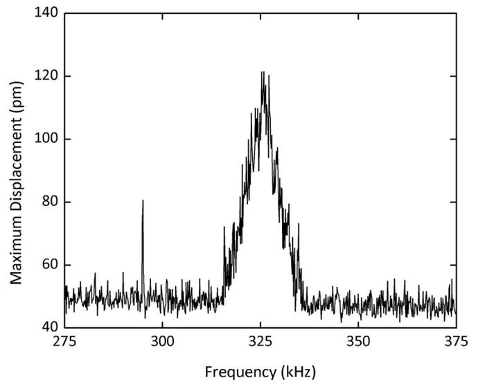
Fig. 9. Maximum displacement of resonator 1 observed within the frequency band around the resonance frequency.
