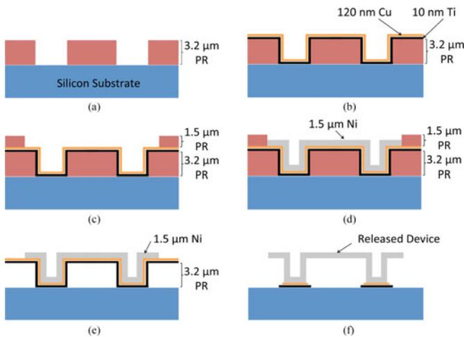
Fig. 4. The fabrication sequence of the MEMS resonator in side view. (a) Photolithography 1, (b) sputtering of titanium and copper, (c) photolithography 2, (d) electroplating nickel, (e) releasing, (f) wet etching.
