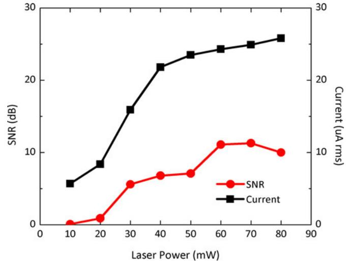
Fig. 6. The change in SNR and the rms value of the PWM current for varying laser power levels.
