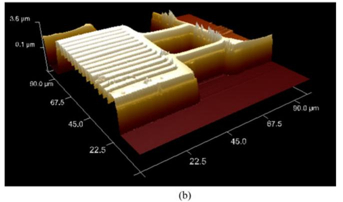
Fig. 5. (a) Micrograph of a released device in top view. (b) Topographic image of the device obtained using an atomic force microscope.
