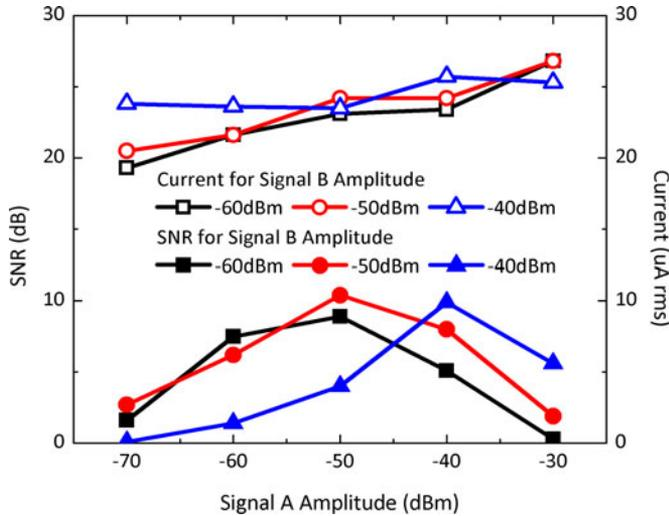
Fig. 7. The change in SNR and the rms value of the PWM current for varying input signal levels.
