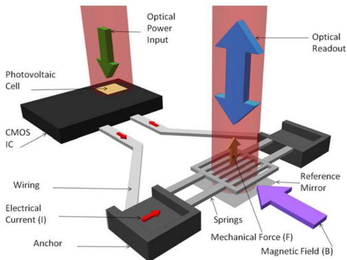
Fig. 2. Main system blocks and representation of MEMS resonator actuation mechanism. Note that the application of diffraction grating interferometry technique would require a reference mirror beneath the resonator structure.
